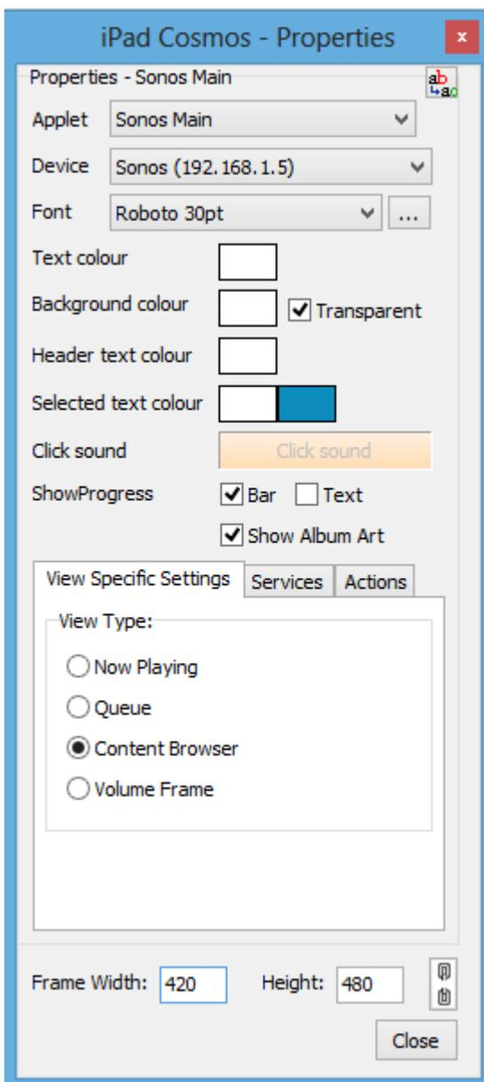
In order to achieve complete functionality, the first three of these types will need to be used in the design, and all need to be the same applet instance. Refer to [Applet Design](#) for more on this. The volume frame offers more fine-grained control over the positioning of any volume control or readout.
