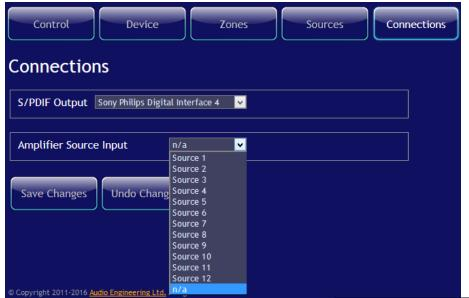
A connection may be setup so that no Axium amplifier input is required. In this case a media player is made available for direct usage of this output and in third party applications it will show the name of the output. This mode would be useful for providing extended media functionality to a home theatre system for instance.
