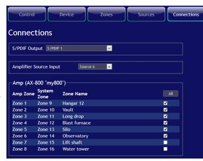
Multiple connections may be defined incorporating the same group of zones. This allows simultaneous media players to be operational on different zones in the mapping at the same time.
