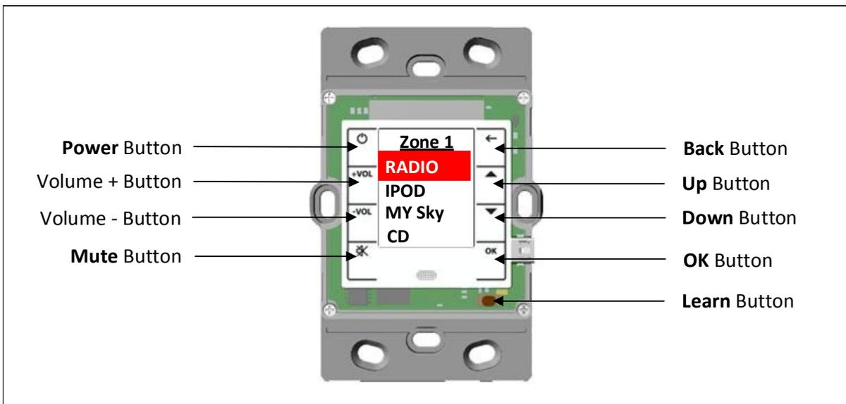
**Step 1.** Connect the AX-KPD keypad as per the instructions to the Axiom system, this will provide power to the AX-KPD keypad and allow you to see the main screen. Fig 1. Remove the cover faceplate from the keypad to expose the learn button Fig 2.
